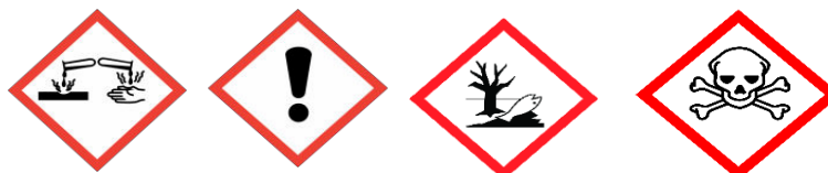
Corrosion Exclamation mark Environment Skull with crossbones
